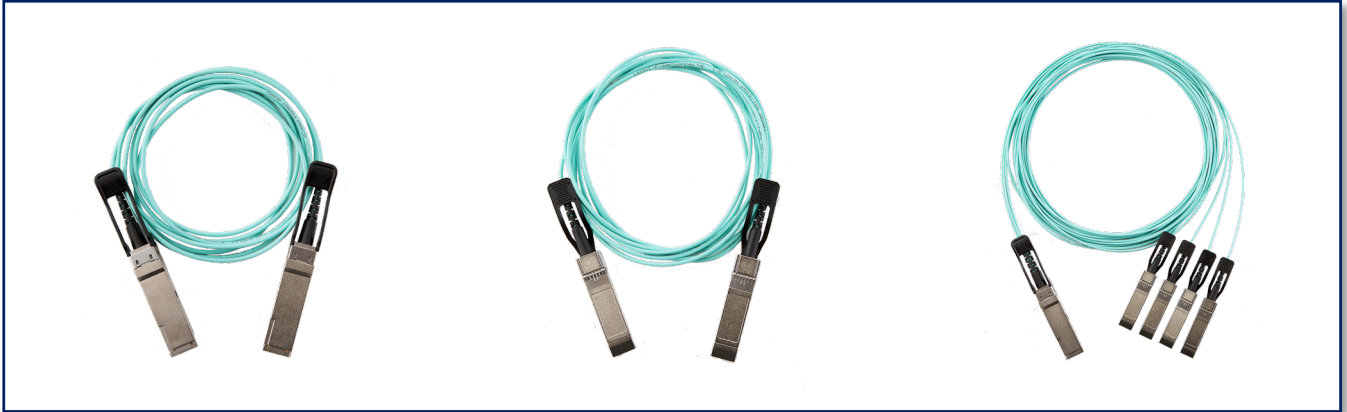
Figure 2 Optomind 28G family products (QSFP28, QSFP28 to 4 × SFP28 and SFP28 AOCs)
